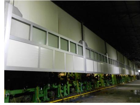
Easy lateral access to hall with lifting doors equipped with motors/ cables.
