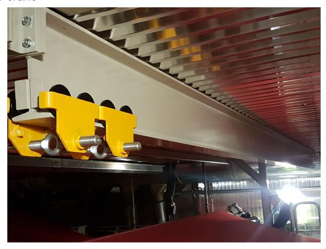
Inner crane with rail for felt change and maintenance operations
