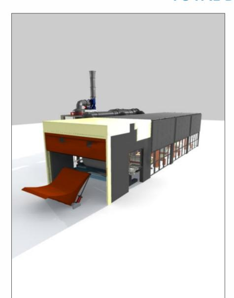
**T Box** (Option) for total winder closure, made by 4 walls and an opening roof:
