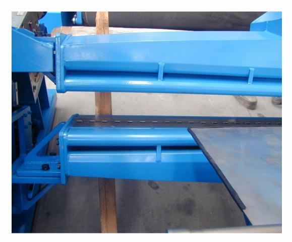
**C Boxes** (Option) are positioned before the rewinding of final jumbo roll to clean across the web the remaning boundary dust:
