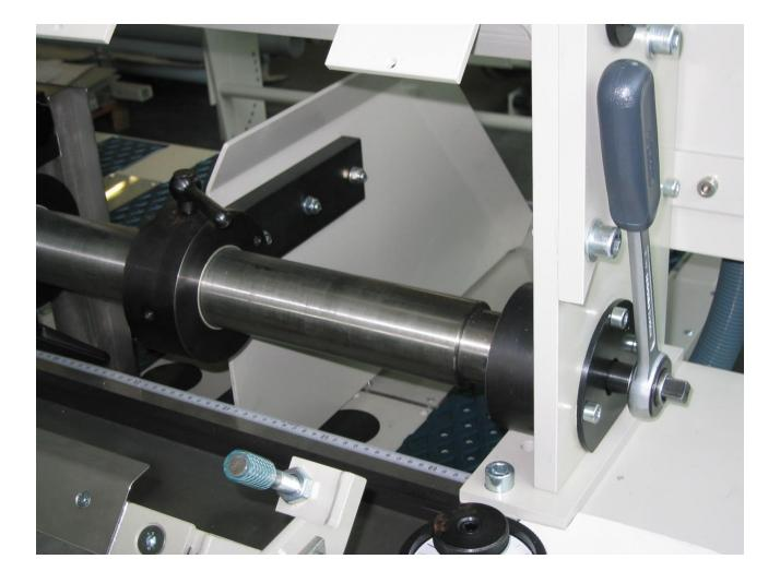
Gluing unit with application and metering (squeeze roller) – made of different material – emergency running property – easy cleaning, short wash-up time
