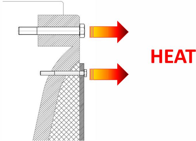
ROTATING YANKEE HEAD INSULATION HAS SEVERAL POINTS OF HEAT LOSS:
