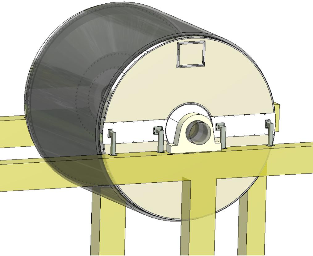
Novimpianti system is composed by a **static element**, filled by high insulating capacity material, fastened to the Yankee dryer's static supporting structure and **completely covering the Yankee heads**.
