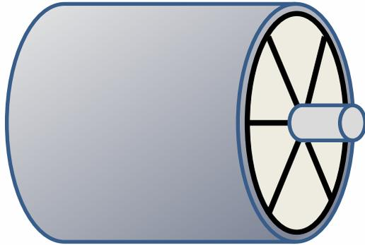
ROTATING INSULATION IS TYPICALLY COMPOSED IN 6 PIECES
