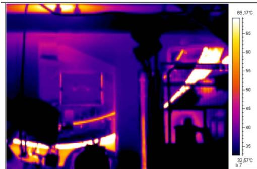
Before installation on Yankee headers surface reached more than 130°C while operating at cylinder steam pressure of 4 barg (159°C). With the installation of YANKEE HEAD SAVERS local temperatures dropped below 80°C.
