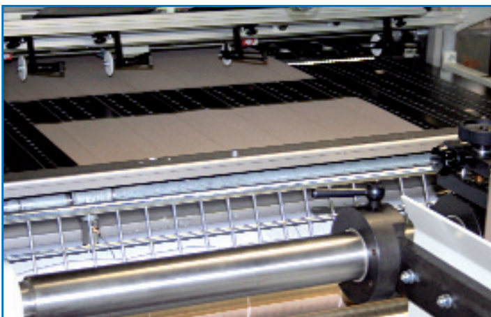
gluing unit with carrier sheet transport
