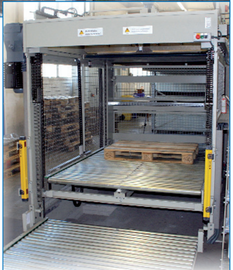
down-stacker with roller conveyor system – suitable for adjusting the position of the pallet in sheet direction
