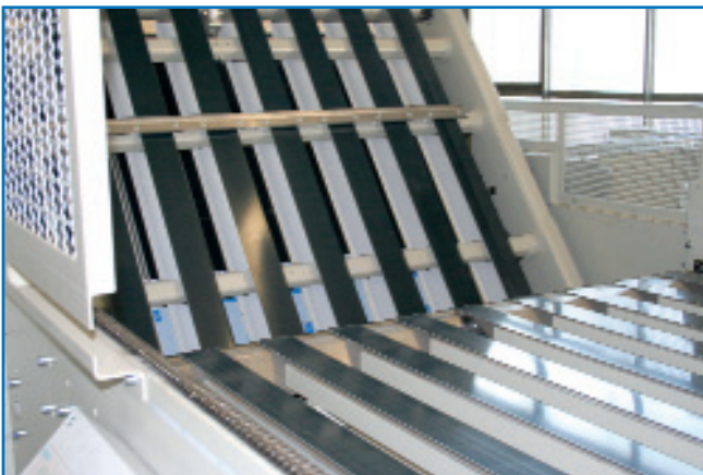
flip-flop (batch-pile turner) – adjustable batch height
