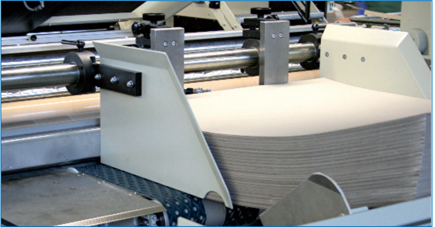
suction feeder model 4R – for non-stop sheet feeding
