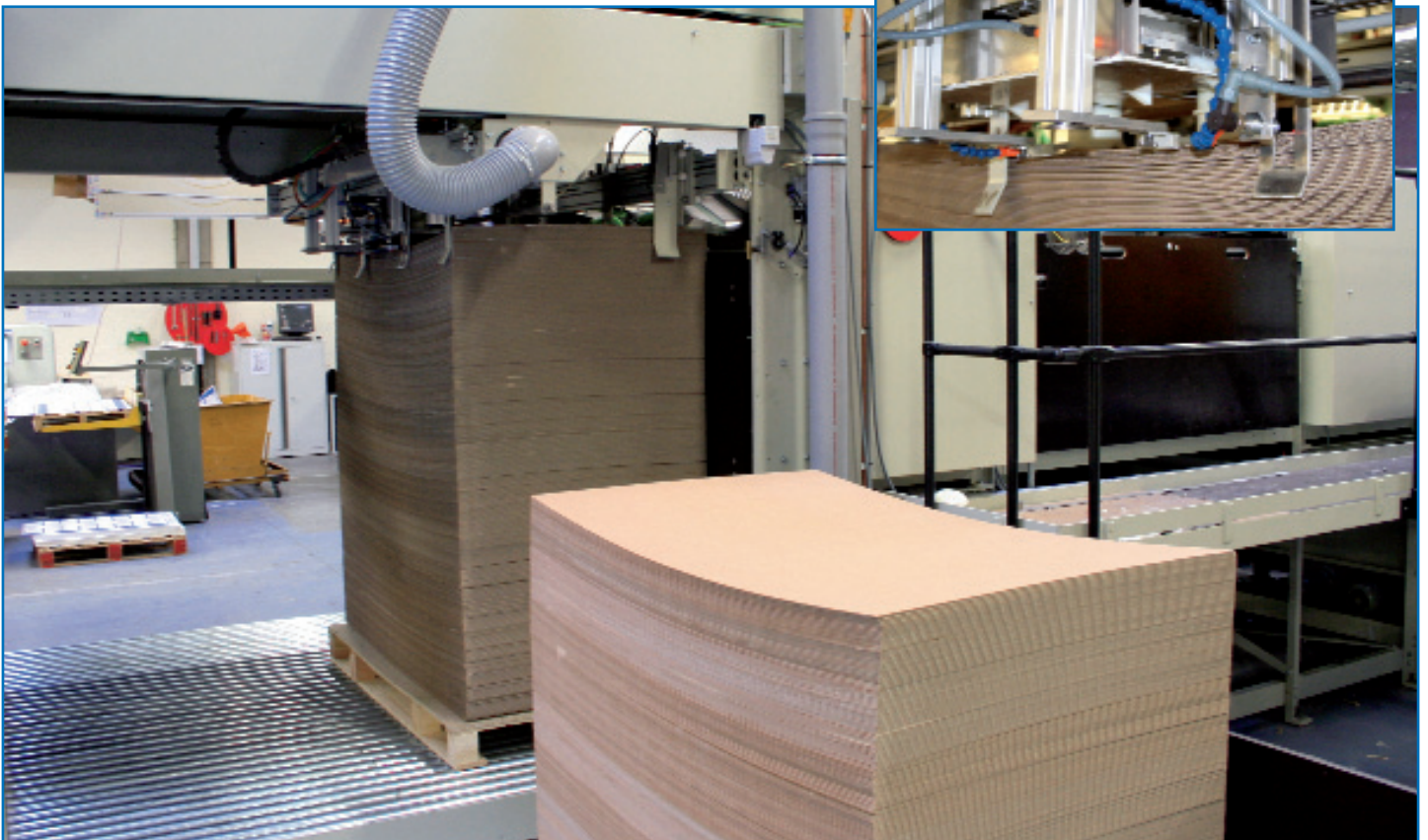
high pile feeder model 4B – with pallet logistic
