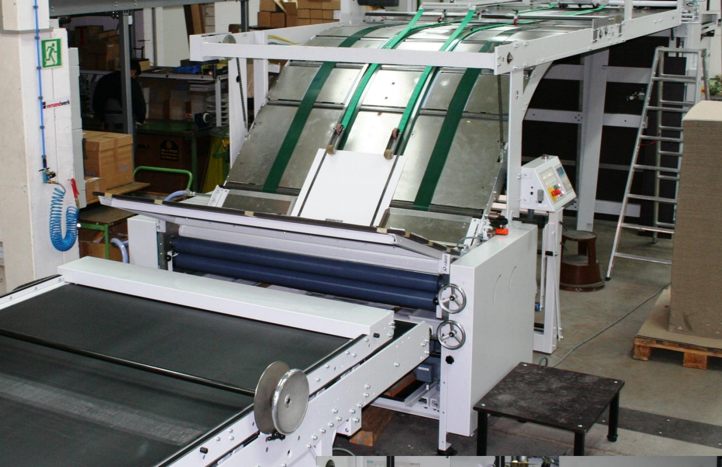
printed sheet feeder with direct driven suction head, as well as motorized sized format setting with digital display
