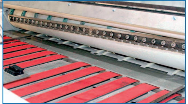
Spiral- / Wendelschnitt helical cut-off knife
