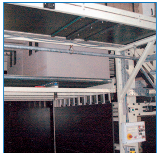
Nonstop-Stapelableger, mit Rollenbahn down-stacker with non-stop operation and roller conveyor
