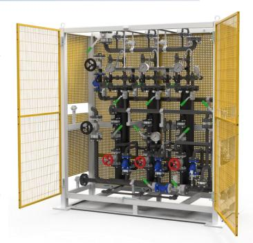
When the level controller detects that the condensate tank has reached its maximum level, the injection valve (VI) opens automatically pumping/pushing condensate, through the check valve in the outlet, back to the condensate recovery unit (CRU). This injection cycle lasts around 5 seconds.
