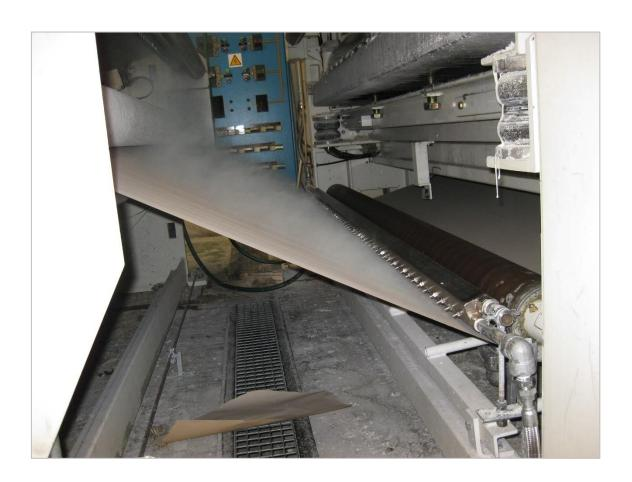
The bond of the two single faces is limiting double wall board production, especially when working with high weight papers such as agricultural grades, since it is very difficult to have heat reach the central part of the board because of the board's self-insulation effect, in opposition to the single facer B-liner bonding that is easily heated by means of the Double Facer's hot plates.
