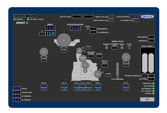
A reliable and versatile **PLC-PLC INTERFACE** with FOSBER's SMART is possible, making possible integration of condensate recovery system into RAS (industry 4.0) and enhanced reaction of the steam pump to:
