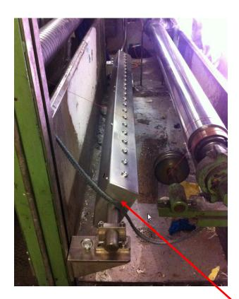
Remoisturizing of Filter Paper before Reeler 2.5 – 3 % Moisture increase profile control 160 g/m2 Filtre paper at 130 m / min
