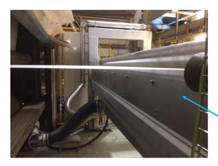
2.7 % Moisture Increasemain purpose moisture profile control2 sigma reduction 1.58 down to 0.18!
