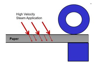
Paper web has an open surface of 80% water, 20 % fiber. The condensation process causes heat and energy transfer **into** the paper with a temperature increase of 10 - 25 °C
