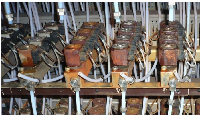
Used Digital valve Blocks Corroded and wearing parts
