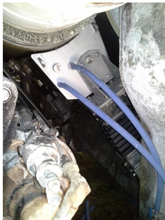
Old VIB Steambox unit replaced by a new W&H Accusteam Steambox reusing the existing control and pneumatic lifting unit
